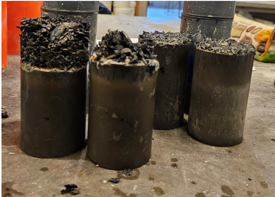
Figure B6: 3% mixtures using large particle size. Since no biochar was truly mixed in to the cement, these tests were discontinued.
